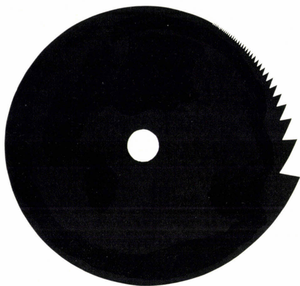
Fig. 13. Disc with edge serrations representing part of the function (15), for experimentally determining the zero points of Riemann's \zeta function.
